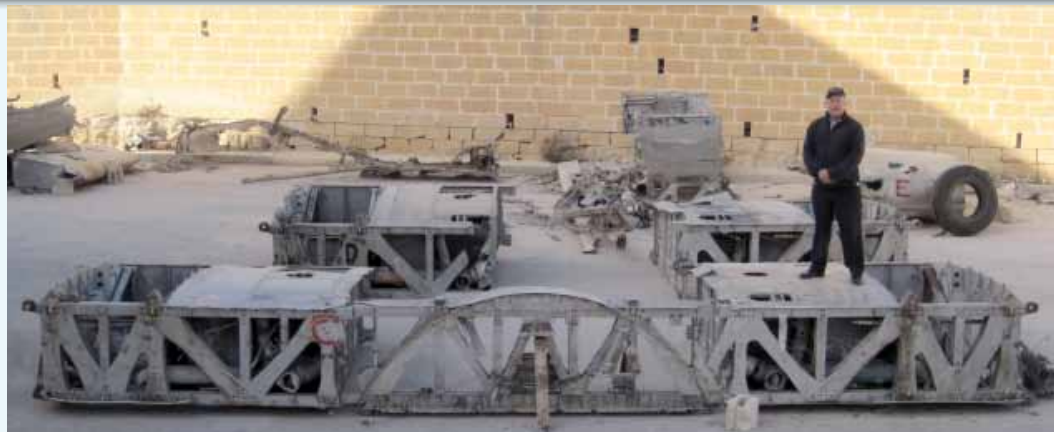
Karl Kjarsgaard at the MHVT compound in Malta in June 2011. All the main wing boxes and centre spar sections are lined up after weeks of disassembly to fit in a shipping container bound for Canada. HP57 Rescue (Canada)
