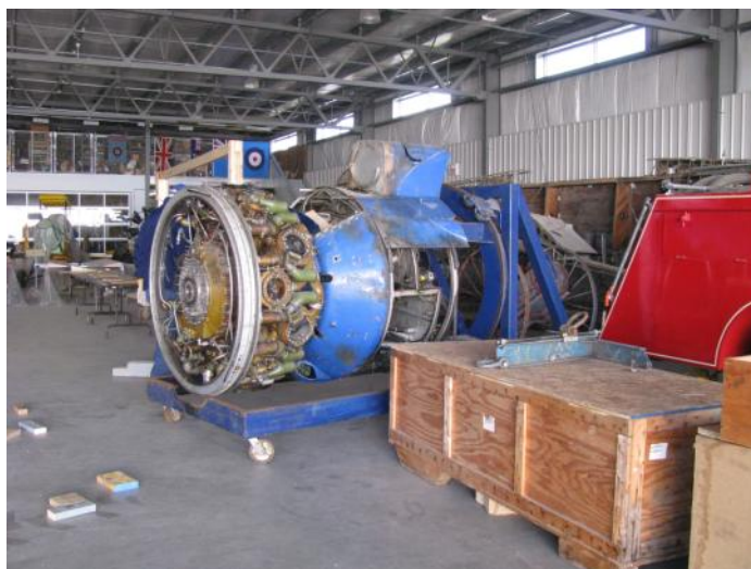
One of the four Bristol Hercules engines in the restoration hangar at the museum
